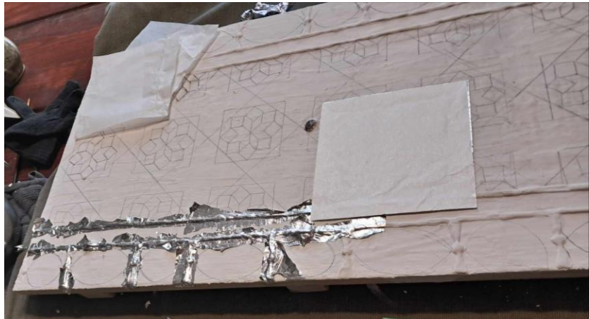
Figure 17 Foil added over entire test board
