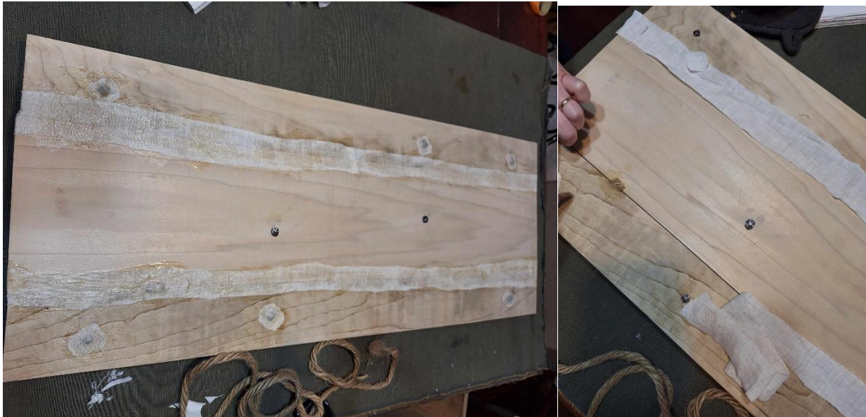
Figure 8 Hole filled with Hemp Fibers
