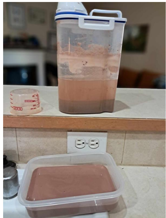
Figure 47 terra sigillata removed from original mixture
